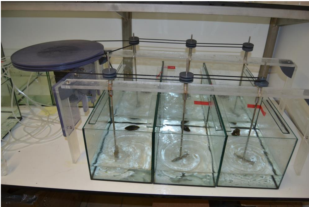
Figure 1. The experimental set-up for measuring clearance rate.
