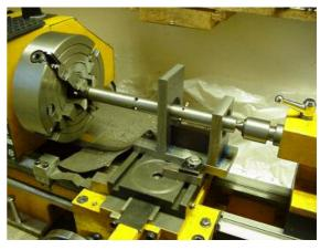
When both pieces has been bored, the frame can be screwed together again and mounted on the crossslide. A dial test indicator can be used to align the frame with the centre line of the lathe, then the holes for the Unimat spindle can be bored out to 35 mm. This way you can make sure the spindle is parallel to the frame. See illustration. I just made a small cutter from 5 mm silver steel (drill rod), and hardened and tempered it.
