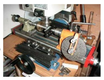
13.0 mm, to give a sliding fit on the Unimat spindle. A 4.2 mm hole wasdrilled in the boss and tapped M5. I then made a slightly tapered 13 mm diameter mandrel and mounted the brass piece on the mandrel. The mandrel was then mounted between the centres and the rest of the worm wheel was finished. Then I could move the mandrel/worm wheel to the old dividing head on the mini mill and cut the teeth.
