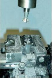
slide was mounted back on the body and locked in position and the two pilot holes opened up to 11.8 mm and reamed to 12 mm. Two 5 mm holes was drilled into the short 12 mm holes, and tapped M6 for set-screws. The set-screw for the long 12 mm hole is M8, and positioned directly opposite the recess for the feed screw nut. The hole (with a diameter of 3.2 mm) continues all the way to the recess, and is countersunk so the small screw clears the reamed hole.
