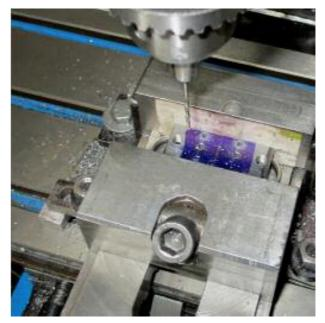
The jig was then used to spot the holes on the under side of the Bearing Blocks – right photo. In the photo the first Bearing Block has been drilled and the last hole in the second Bearing Block is about to be drilled (2.5mm).
