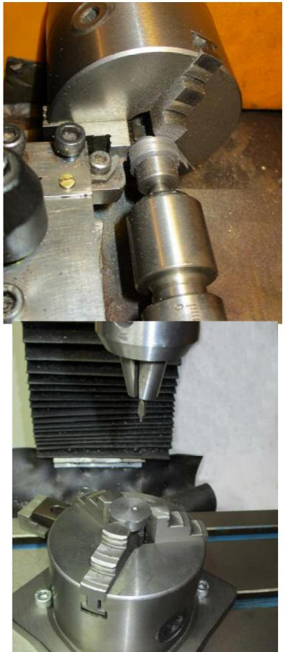
The Eccentric Strap was fabricated from a piece of steel tube with 18mm I.D. from my scrapbox. I silver soldered a piece of mild steel to the tube, and drilled a 2.5mm radial hole in the mild steel piece and tapped it M3 for the Eccentric Rod.
