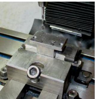
After drilling and tapping (M3) the holes in the Bearing Blocks the blocks were clamped to the jig and the jig mounted on an angle plate on the lathe faceplate, and the hole for the Crankshaft bearing drilled and bored – left photo. I clamped a piece of steel rod opposite to the angle
