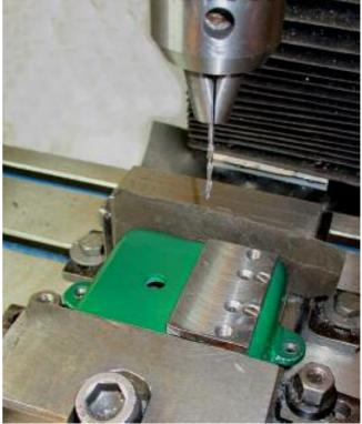
the 8mm reamer through, it barely made some swarf, the left photo show Bearing Blocks and Crankshaft in place. The Crankshaft turned easily in the bearings.
