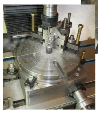
Before parting off the work was mounted on a rotary table and the ends rounded – above photo. The finished part is shown to the right.
