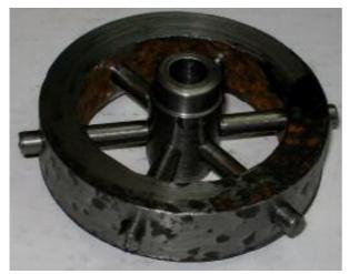
Then all joints were fluxed and I silver (hard) soldered the parts together. The flywheel was a bit wobbly after the soldering so I mounted it on a between centres mandrel so I could turn the outside and sides – see right photo.
