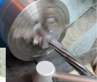
To be able to turn the spigot on the underside of the Bottom Cover I first used the Bottom Cover to spot the holes on the bottom end of the cylinder (while still clamped in the 4-jaw) – left photo. I could then use my Dremel clone and drill four
