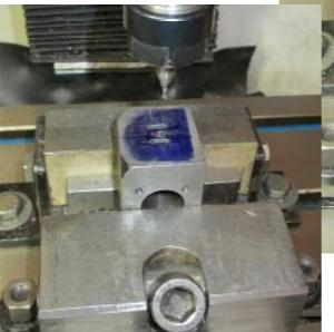
I then used a 1/16" slot drill to mill the two narrow ports
