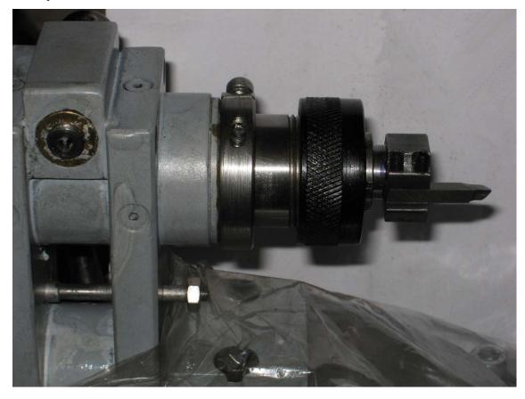
The holder for the 1/8" HSS tool bits worked so well that I decided to make a similar holder — though a bit larger — for the 5mm square HSS tool bits I use in my small lathe. I found a suitable piece of mild steel in my scrap box and first squared it up in the milling machine, and then mounted it in the 4-jaw so I could turn the 12mm shaft — right photo.
