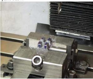
Since I milled two slots, two of the tapped holes for the set screws used to clamp the tool bits, had to cross. I drilled a small pilot hole first, then used a larger 3.3mm drill for the cross-hole. After tapping the large hole M4 the small hole was opened up to 3.3mm and tapped M4. This seemed to work fairly well and the holes ended up where I wanted them. After tapping the last hole I cleaned up the previous hole the remove swarf.
