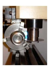
The collet was turned from a piece of 40-mm diameter steel rod about 20-mm longer than required. The extra length was used as a chucking piece. After centering the hole was bored to 25-mm and the outside turned slightly oversize on the tapered part (right picture). The part to receive the thread was turned to size and threaded with a 1.25-mm pitch. The collet was then partly parted off and I used a hacksaw to cut
