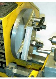
While the two pieces was clamped together I drilled a 4-mm pilot hole for the index pin. I made a small distance piece tapped M4 and used this to clamp the two plates together while silver soldering. I put thin pieces of paper around the distance piece and oiled the screws lightly; these turned into carbon during heating so it was easy to
