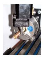
3-mm diameter pilot drill, and I used a ½ in. end-mill to open up the hole to final diameter (right picture). Because a thinwalled tube was used I could not use a twist drill over 5-mm without breaking into the inside of the thinwalled tube, so I had to use an end-mill.
