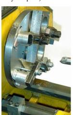
drill, I could the use the tailstock centre to push the work against the faceplate when clamping the plates to the faceplate (see picture to the right). I used two pieces of brass as shims between the work and the faceplate and four clamps (in the picture to the right the two last clamps are not yet in place). I bored the holes so the steel tubes would slide in easily (about 0.1-mm clearance for the silver solder). See picture to the left.
