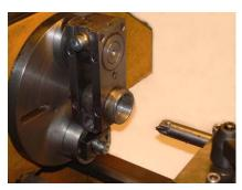
could adjust the tension so the tool holder and the fixture could be knocked around a bit with a plastic mallet. This way I could adjust the position of the spindle tube and get a runout of around 0.1-mm using a Dial Test Indicator (right picture).
