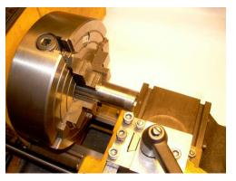
piece from a 38-mm steel rod was used to make a closing nut for the Myford collets, and a 7-mm thick collar with a 25-mm diameter hole. The collar is split and a M4 socket head screw is used to clamp it around the spindle. The closing nut was knurled on the outside and two holes drilled on the front. The two holes in the front are used by a small spanner. The nut was heated and treated with vegetable oil to give it some rust protection.
