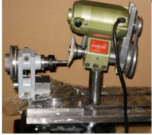
The various parts were mounted together – see left photo – and I ground the end teeth on an 8mm endmill.
