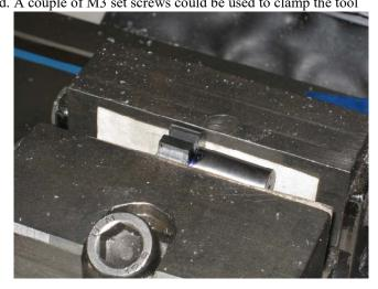
Below is a photo of the holder mounted in a 12mm collet and with a 1/8" HSS tool bit.
