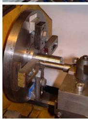
to bore the hole for the tailstock center).
