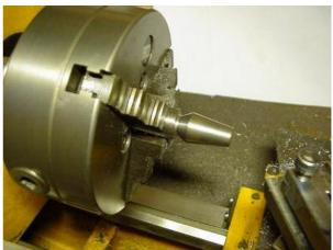
Finally I mounted the collet I had made in the fixture and milled the slots. I put a piece of mild steel rod in the collet so the clamping force wouldn't deform it.
