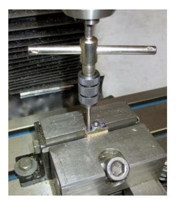
The two parts were held together with some M3 screws and the position of the 8mm hole was marked out and a pilot hole drilled. This hole was opened up to 7.8mm and then reamed to 8mm – right photo.
