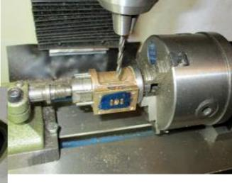
The photo to the left shows the steam chests mounted, I still need to drill some holes for letting steam into the steam chests.
