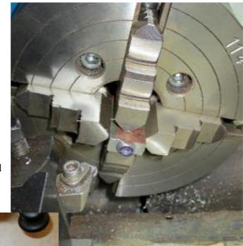
Next I used a small hacksaw to saw the 12mm square brass in two and mill the sawn surfaces flat – left photo.
