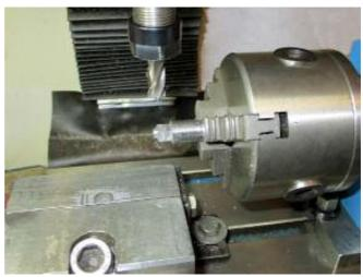
Two holes were drilled at 90 deg and a bit offset. One 2.5mm hole and one 3mm – right photo.
