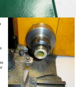
The next operation was to mill away the sides to make the apertures on each side of the Trunk Guide, I used an 8mm end mill.
