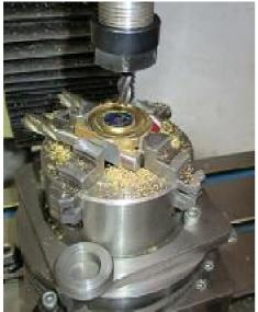
test the fit of the spigot that will enter the bottom of the Cylinder. I also plan to drill 6 holes spaced 60 deg. apart on a 24mm PCD so I can use the ring as a drill jig.
