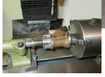
After soft soldering the brass flats to the Port Faces of the Cylinders I marked out positions in each corner and drilled a 2.5mm hole through the brass flat and around 4mm into the Cylinder. The holes were then tapped for M3 studs (well, pieces of threaded rod) – left photo.
