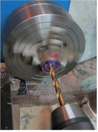
The Bottom Cylinder Cover was then fitted and oriented in the correct way with respect to the cylinder port face and I used my Dremel clone rotary tool to drill a 2.5mm hole in the cylinder end – right photo. I tapped the 2.5mm hole M3 and used a cheese head screw to hold the cover in place when drilling (and then tapping) the next hole. With three holes drilled and tapped I could secure the cover to the cylinder and face the spigot of the gland and drill and
