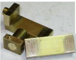
Even then the parts moved a bit while silver soldering/brazing the parts so may be small brass screws next time, the photo to the right shows one of the brazed Steam Chests after pickling and a few strokes with a flat file on the underside.
