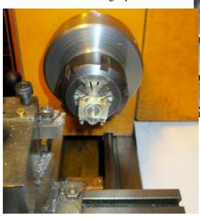
I then clamped a piece of 12mm mild steel rod in the lathe and turned a short spigot to a diameter just over 8mm so I could clamp the split bearing onto that part of the rod- photo above.
