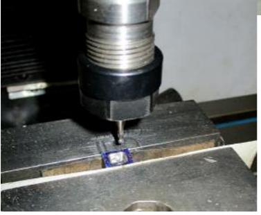
The parted off valve was mounted in the milling vice and a 2mm slot drill used to mill the cavity to dimensions using the handwheel dials – left photo.
