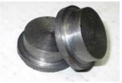
The straps were fabricated from two short pieces cut from a steel tube with 18mm I.D, and 22mm O.D. I silver (hard) soldered two small pieces of mild steel to the tube pieces. I will drill a 2.5mm hole in each and tap M3 for the Eccentric Rod – right photo.
