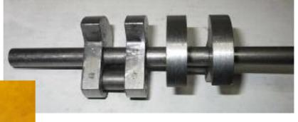
Crankshaft and inserted some mild steel pins together with a drop of anaerobic glue. The Crankpins were "pinned" in the same way. When the glue had cured I used my Dremel clone to grind the pins flush – see photo above.
