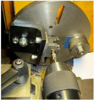
as the split bearing, to make sure all three holes for the Crankshaft ended up at the same height. The holes in the two blocks were bored to just under 10mm so the pieces of 10mm OD brass tube was a press fit in the hole. The brass bushes were then reamed to 8mm. The brass bushes were made over length, and the blocks were mounted again on the faceplate jig and
