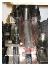
The next operation was to mill the dovetail. The work was clamped to the milling table with four clamps (one in each corner) and a dial test indicator used to align it. First a slot was milled with a carbide tipped mill I made a long time ago (left picture). This slot is a bit wider than than the diameter of the carbide tipped dovetail cutter I made for this project. The steel was hard and I had to take light cuts using a slow feed to
