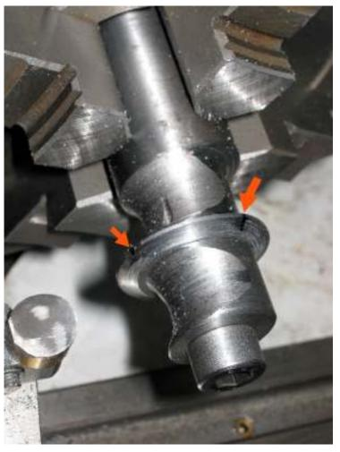
The cutter is then mounted on an arbor in an indexer, and then the part in front of the "high spots" on the cutter blank is milled away the inner corner is filed round with a small round file. The cutter is marked with module number and for how many teeth it is intended, and heated to bright red and quenched in water, then tempered to straw.
