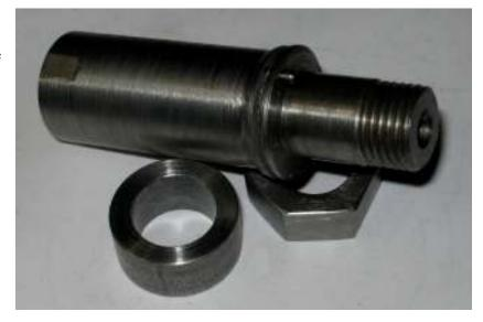
the bottom of the 2mm hole. This means that when the cutter blank is clamped on the mandrel the pin is slightly pressed down into the hole.
