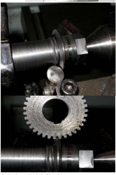
Making Gear Cutters with 4 Cutting Edges - 7 -
