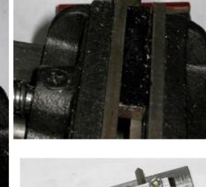
I also drilled a 4 mm hole and made the "nut" that clamps the tool-bit in the slot.
