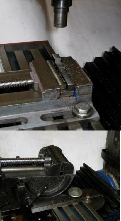
This way I could mill the side of the tip of the toolholder (right photo). And with a 3mm end-mill mill the slot for the tool-bit (photo below).
