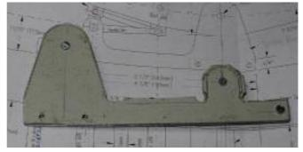
as a jig to drill corresponding holes in the second piece. The two pieces were bolted together using two small screws and then the other holes could be drilled through both pieces, as advised by Rudy. I used a file to file the parts to final dimensions.
