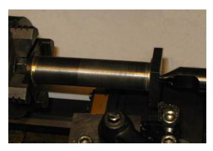
bicarbonate to neutralise the acid. Then the work was mounted in the lathe and the ends faced. I also turned the inner part of the *Entablature* to get a nicer transition towards the column. I used the holes in the *Spring Beams* to spot the corresponding holes in the Entablature and drill 2.5mm and tap M3. The matching holes in the *Spring Beams* were opened up to 3mm.
