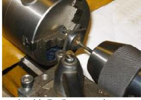
four 3mm holes 90 deg. apart in the Top Cover and used the Top Cover to spot the corresponding holes in the Cylinder top face. The four holes in the Cylinder were drilled 2.5mm and tapped M3.
