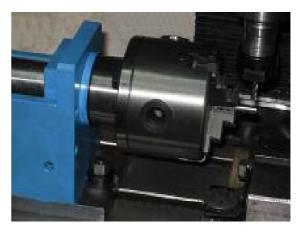
6mm dia. mild steel rod. The (over length) work was held in the 3-jaw on my indexing head and one side milled down 1mm for a length of just over 8mm. Then rotated 180 deg. and milled the same way. Then over to the lathe and the work was parted off to just over finished length, faced and centre drilled and drilled 2.5mm and tapped M3 for the *Piston Rod*. Then a 1.6mm hole was drilled from the front and into the hole for the gudgeon, and tapped M2.
