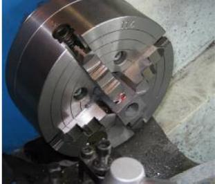
I rotated the work in the 4-jaw so that the *Port Face* was facing outwards and small curves were turned at the top and bottom just to make the Port Face stand out a bit.
