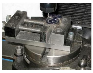
The hand-wheel dials on the milling table was used to place the cutter 7.5mm from the centre of the 4mm pivot hole when milling the steam channels, and the 17.5mm distance to the 2.5mm hole that will be tapped M3 for a screw to hold the Little End of the *Eccentric Rod*.
