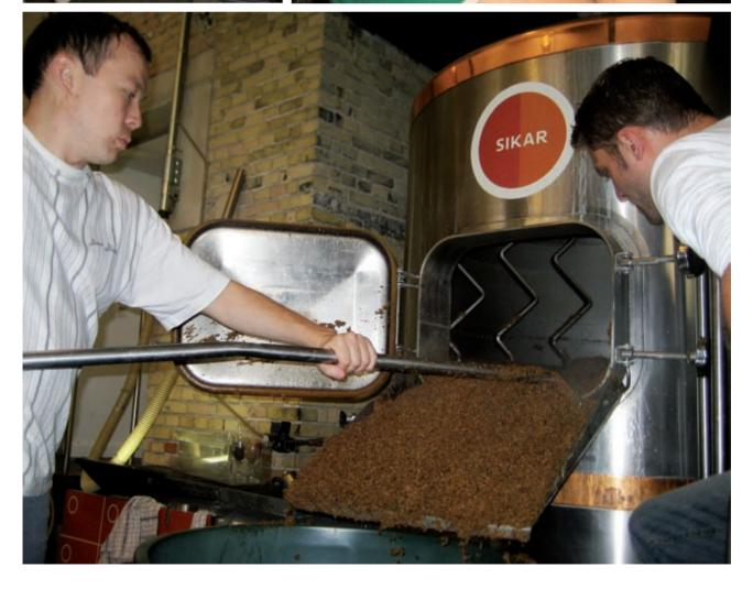
Mashing-in could commence and after the saccharification check, run-off to the lauter tun could start. Samples for wort strength were taken with short intervals to ensure extract yield of last runnings and wort strength in the wort kettle. Other students had calculated the amount of hops pellets to add to the wort kettle, based upon alfa-acid contents in the hops used and on the microbrewery's utilisation degree of hopping.
