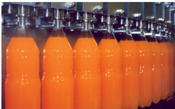
The Innofill DRV is the filling system of choice. It is a computer-controlled, volumetric filling system which handles carbonated and non-carbonated beverages.
