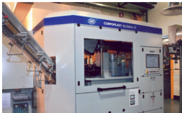
An InnoPET Blomax stretch blow molder produces PET-bottles in the new non-refillable PET bottle line.
