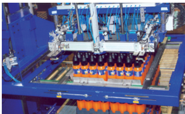
In the next step, the Innopal RS3 column-type palletising robot grasps a layer of single bottles using a packing bell and places it on the displays.
