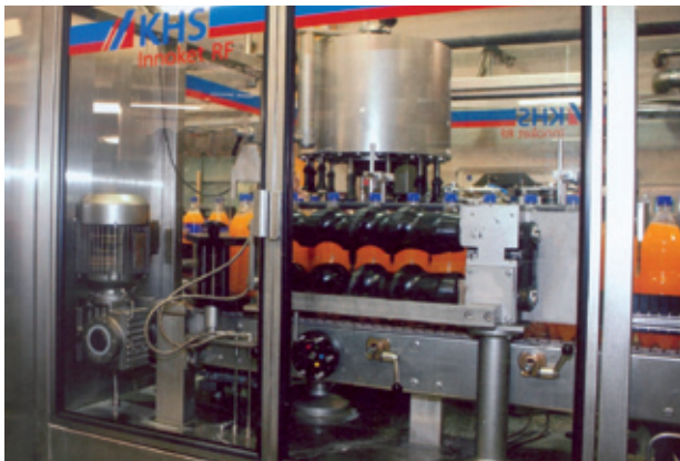
An Innoket RF 25 roll-fed labeller handles the wrap-around labelling of the PET bottles.
