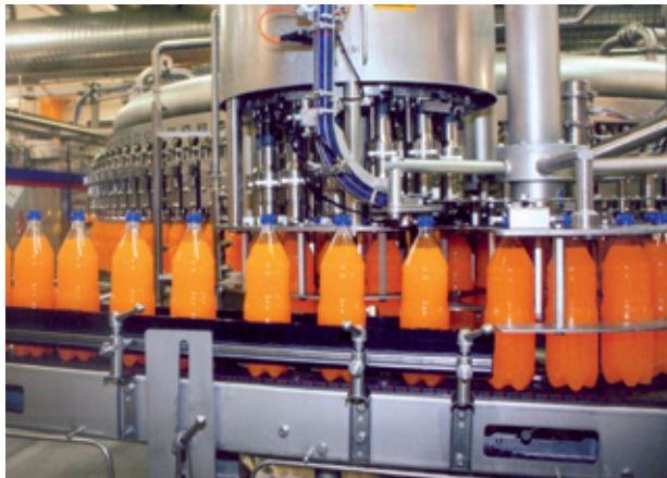
The Innofill DRV filling system is monoblocked with an Innofill SV-ACF. The screw capper features an uncomplicated open, hygienically designed structure and a constant capping force, which makes opening more convenient for the consumer.
