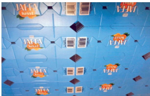
It is possible to also position cardboard layers onto single PET bottles before placing them on a new display. This makes it possible to produce double top packs for 1.5 and 2.0-litre non-refillable PET bottles.
