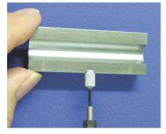
Chamfering of aluminum workpiece
