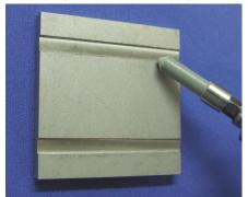
Breaking edge of steel workpiece
