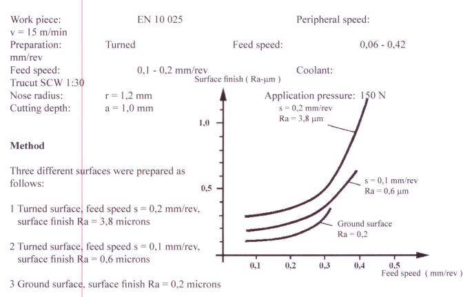
These surfaces were polished at various feed speeds. The graph shows the surface finish as a function of feed speed.
