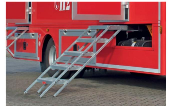
■ **STOWED TO SAVE SPACE:** Steps can be easily pulled out. Space-saving arrangement thanks to simple folding mechanism in the vehicle.
