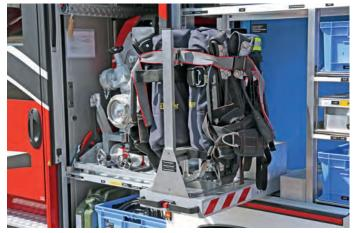
Two additional devices are placed easily removable on a pull-out in the equipment room in addition to two respiratory devices lorried in the crew room.
