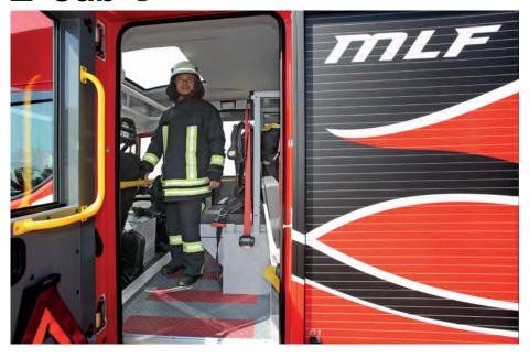
The standing height impressively illustrates the spaciousness of the cabin. The seats at the door openings automatically provide the optimal movement space during entering and exiting.
