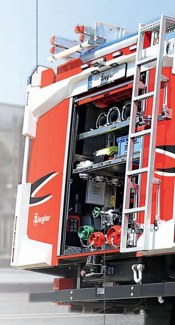
Clearly arranged and ergonomically optimized pump control station. Proven Z-Control
