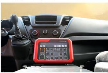
The machine operator and the group leader can view and control all important functions through the Z-Control operator panel that is placed rotable at the instrument panel. The ergonomically designed control elements are constructed clearly and clearly arranged.
