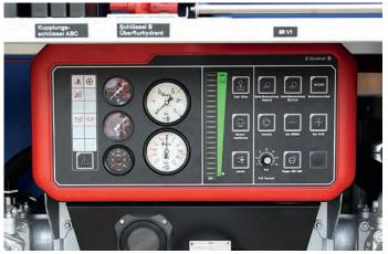
The ZIEGLER pump control station convinces through its very clear and operator-friendly structure. The machine operator has a view of all functions on the Z-Control operator panel. The large buttons are designed glove-conforming.
