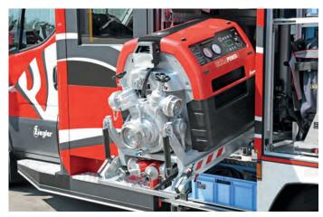
The heavy load extension for the portable pump can be lowered. Due to its diagonal position, the device can be removed quickly, ergonomically gentle and unhindered.
