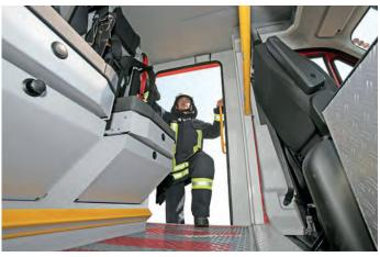
Individually configurable: Each individual seat can be equipped with drawers, flap chutes or commercially available plastic boxes.
