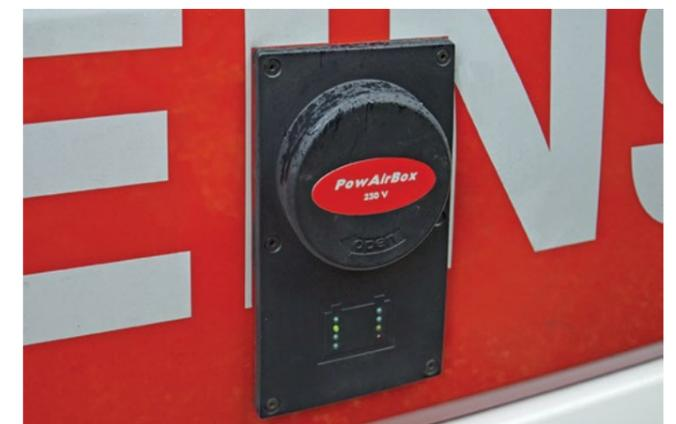
■ **POWAIRBOX:** The combined power and compressed air supply with automatic eject. Infeed possible with 230 V.
