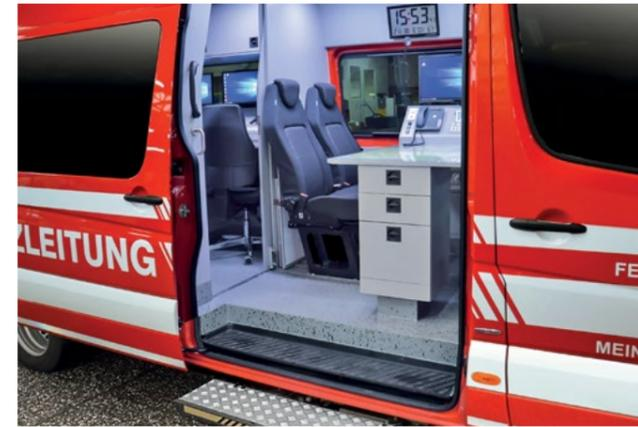
■ **DIGITAL:** Communication is everything – the latest radio and telecommunications technology supports emergency personnel so that they can quickly resolve the situation. Equipped, among other things, with state-of-the-art digital radio and equipment with 2 meter and 4 meter four-channel radio, two command stations with data connection linked to the control center guarantee optimum communications between the individual emergency personnel. Quick organization – quick success.
