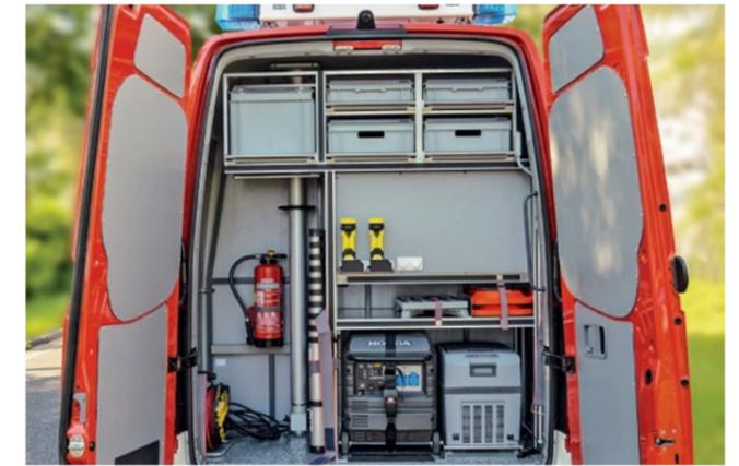
■ **EVERYTHING WITHIN REACH:** Equipment ergonomically loaded in the vehicle's rear ensures a quick and safe removal.
