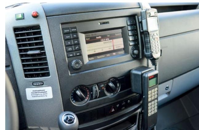
■ **DRIVER'S CAB:** Ergonomic integration of radio and telecommunications equipment in the driver's cab.
