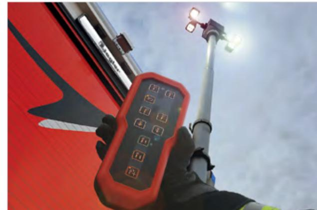
**Light mast / Z-Control-Light mast control**
